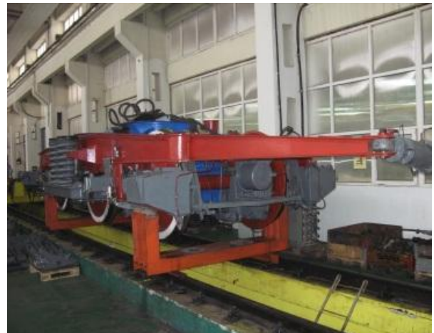
Bogies burn test stand
